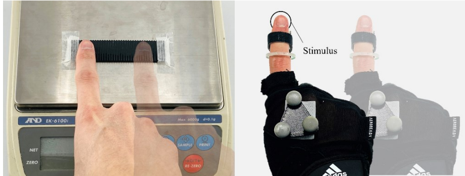
Fig. 6. Experimental Scene. Participants initially traced the 1D grating plate (right) to feel its texture, then donned the device and assessed the presented stimuli (left).
